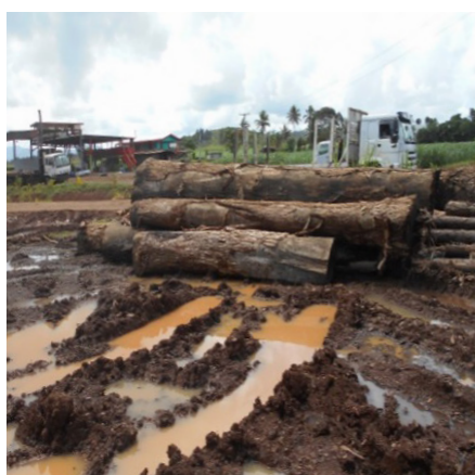
Figure 9: Log yards not in good condition and logs piled on the ground without proper bearers. This was one of the most common practice by most sawmills in Fiji. A well maintained yard with proper bearers will protect logs from blue stain and other defects and reduce sawmill losses.
