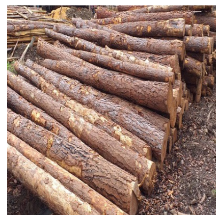
Figure 9: Log yards not in good condition and logs piled on the ground without proper bearers. This was one of the most common practice by most sawmills in Fiji. A well maintained yard with proper bearers will protect logs from blue stain and other defects and reduce sawmill losses.
