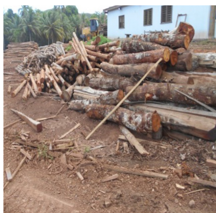
Figure 9: Log yards not in good condition and logs piled on the ground without proper bearers. This was one of the most common practice by most sawmills in Fiji. A well maintained yard with proper bearers will protect logs from blue stain and other defects and reduce sawmill losses.
